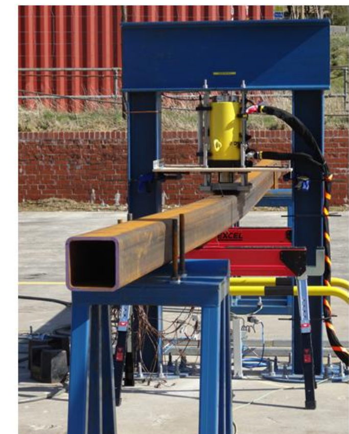
Square hollow section (SHS) under bend load (pre-CO 2 release)
